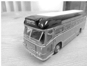
This was developed by Midland Red to coincide with the opening of the M1 motorway in 1959 and provide an express service between the midlands and London. It had an 8 Litre Turbocharged engine and reportedly reached over 100mph at a time when family saloons struggled to top 60mph. The M1 had no speed restrictions until 1967 when the 70mph limit was introduced.
